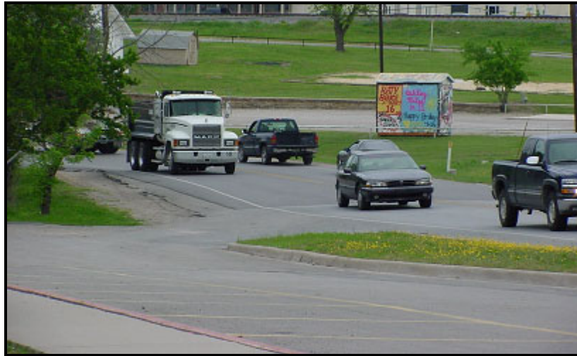
Figure 8. Site with Driveway Located near Horizontal Curve – Inadequate Sight Distance.
