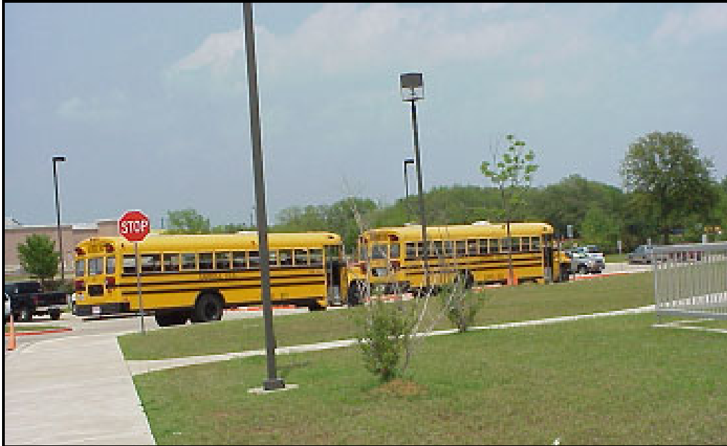
Figure 14. School Buses Staged in Preferred Method – Single-File Right Wheel to the Curb.
