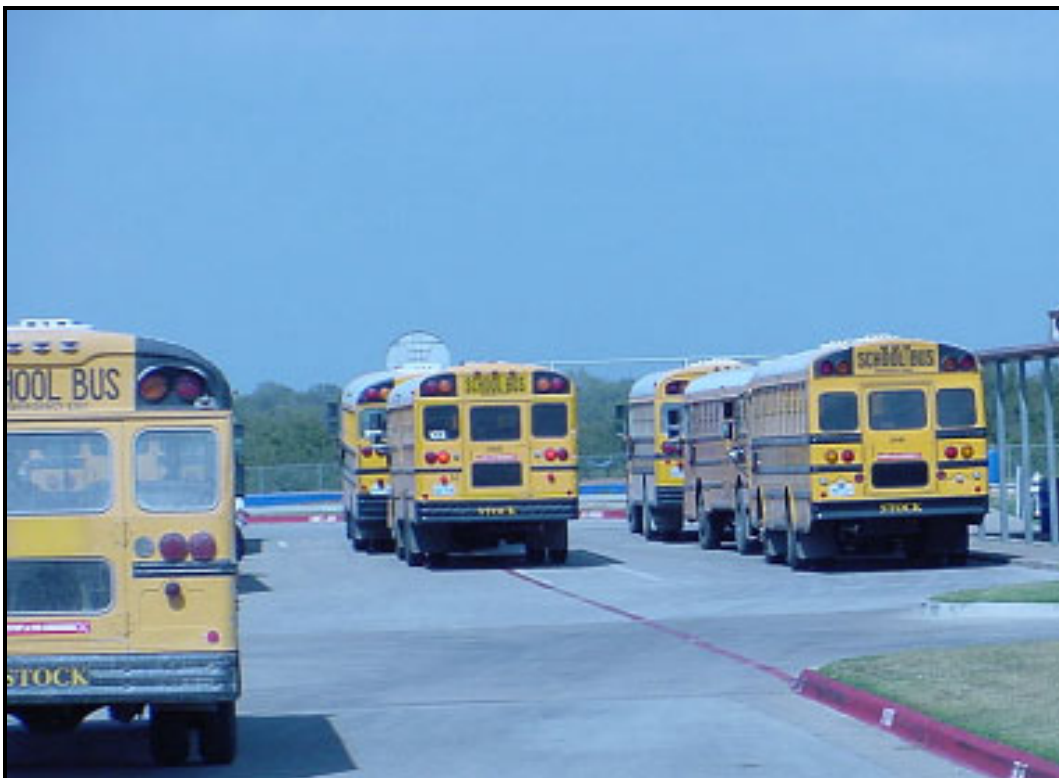
Figure 15. Buses Staged in Multiple Columns – Avoid if Possible to Reduce Potential Conflicts.
