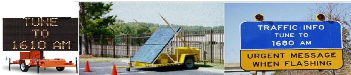
Figure 3. Portable HAR and Portable and Static Signage for HAR (10)
