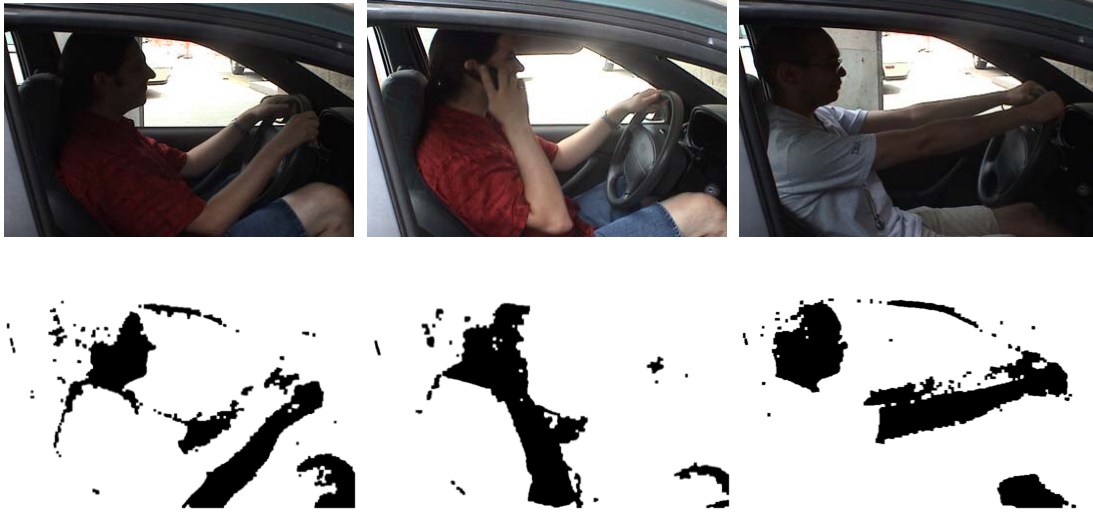
Figure 2.1 Skin color detection (bottom row) on various images (top). Skin color is indicated in black. The results are post-processed by a sequence of morphological erosions and dilations.
