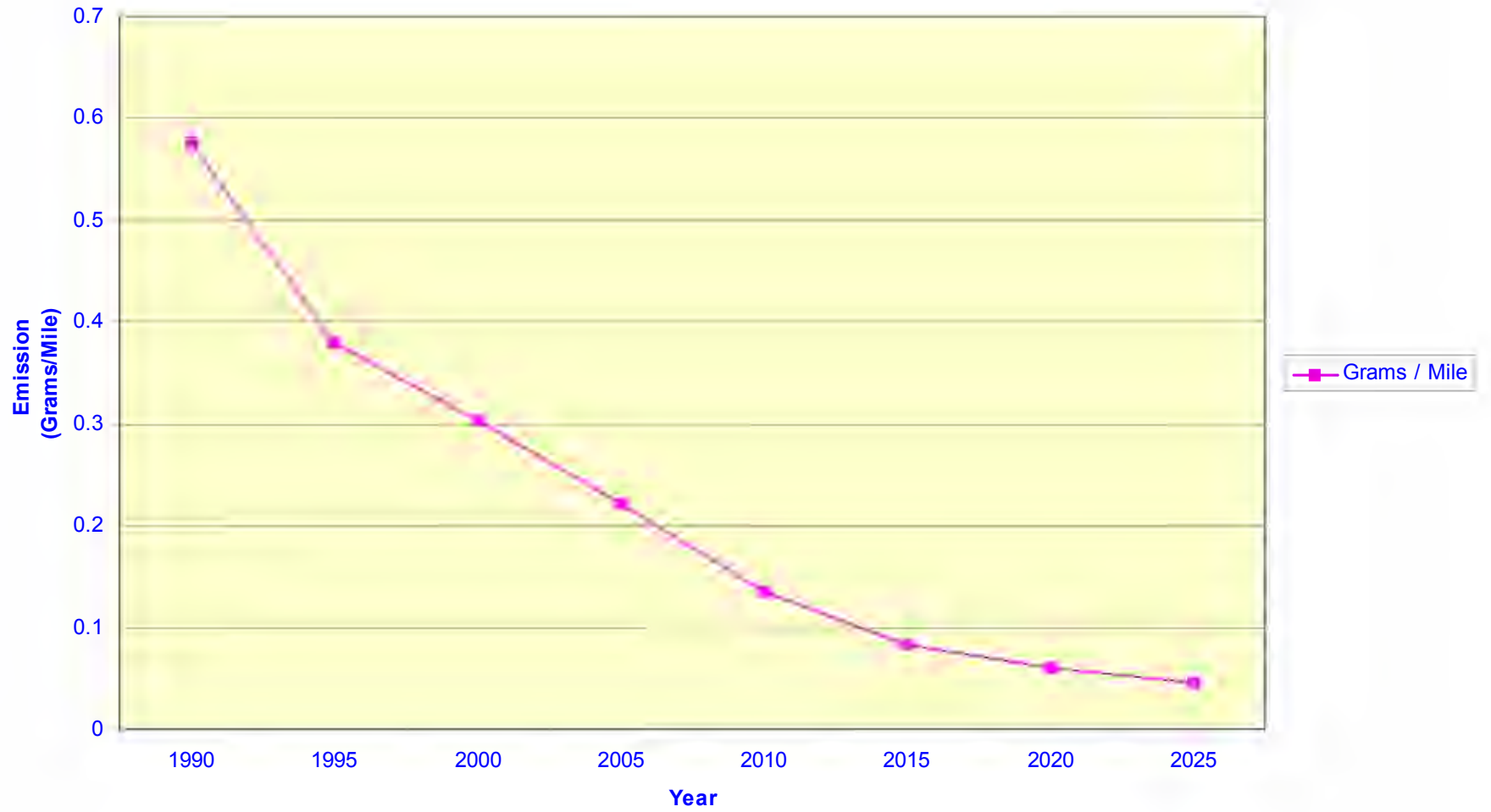
FIGURE 1 - PM10 EMISSION FACTOR TRENDS FOR HHDT EMISSION vs. YEAR (1990-2025)
