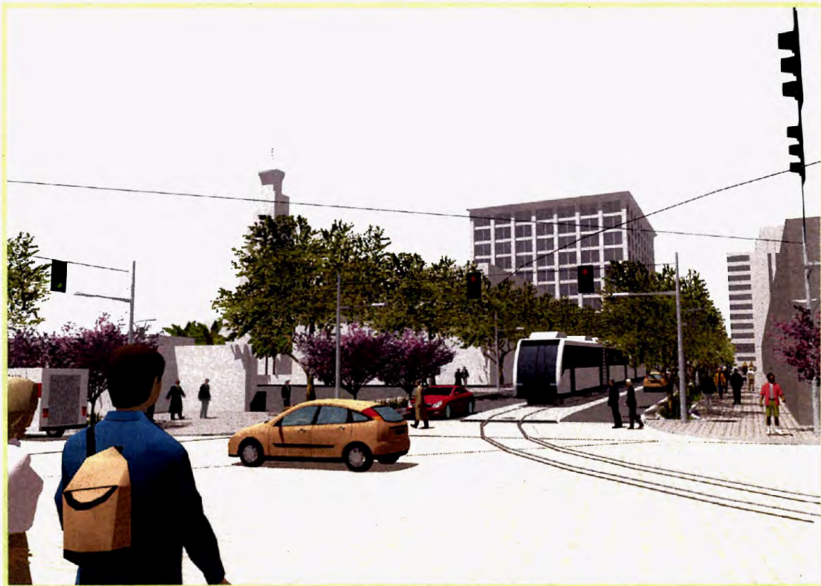
Trains running at-grade will have to traverse some parts of the At-Grade Emphasis LRT Alternative alignment slowly to navigate 90-degree turns and avoid conflicts with automobiles and pedestrians.
