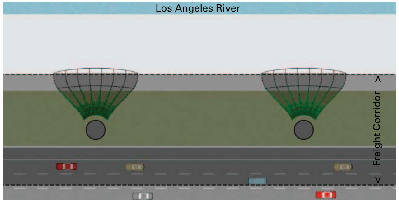
Plan view of green screen near L.A. River, which allows for Caltrans inspection of structure
