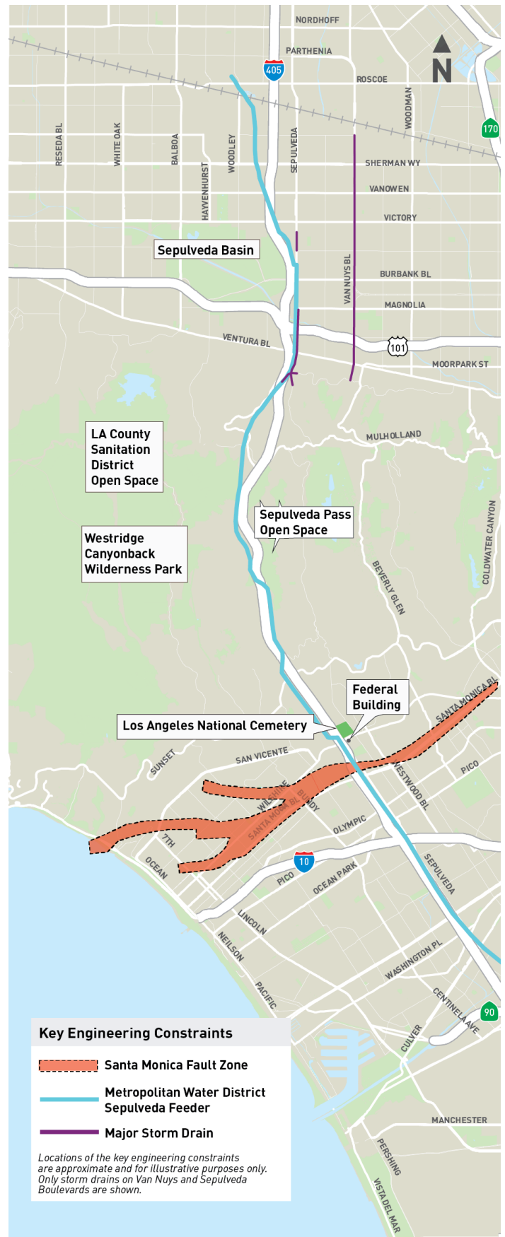
Figure 5-2. Key Engineering Constraints
