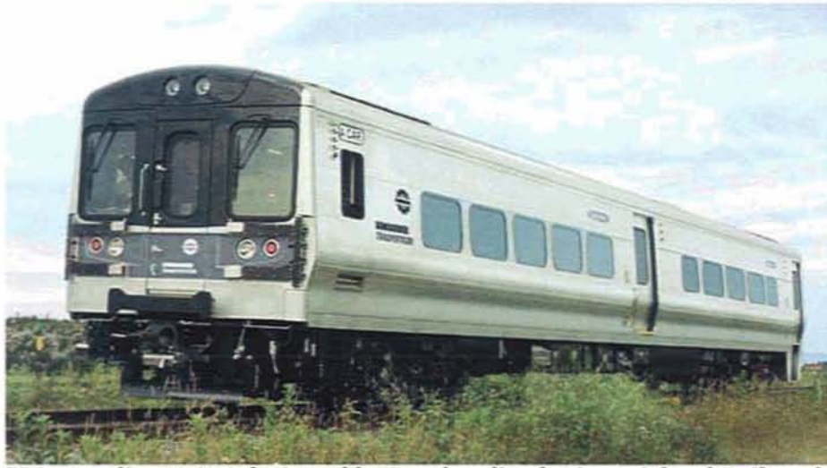
FRA compliant DMU designed by Bombardier for Long Island Railroad and Oregon Department of Transportation
