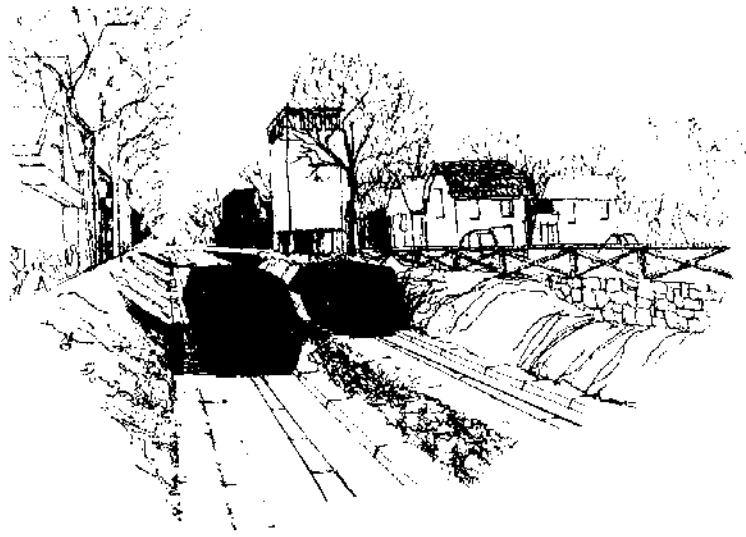
Automated guideways may be depressed—as in this parkway adjacent to residential areas—at grade level, or elevated to suit the locale of the installation.
