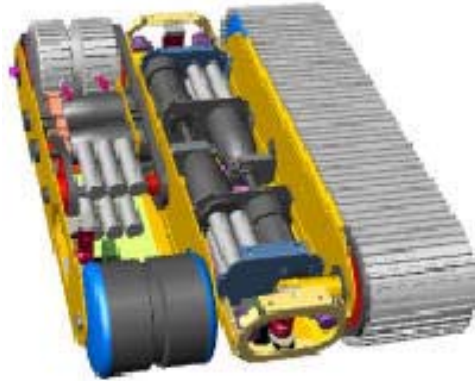
Figure 3. Cutaway of the Novel UGV showing components.
