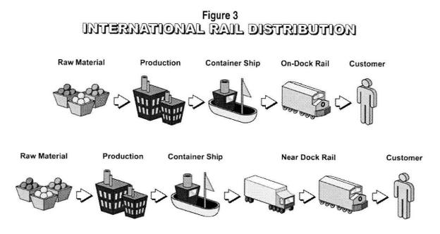
As shown in Figure 3, international goods arrive at the Ports via oceangoing vessels and then leave the region via rail. Sometimes the cargo is first loaded onto trucks for transport to inland (near-dock, off-dock, or inland distribution centers) for transloading to rail. These goods move to points east of the MCGMAP region (typically distances of 500 miles or more) and are shipped as whole containers.
