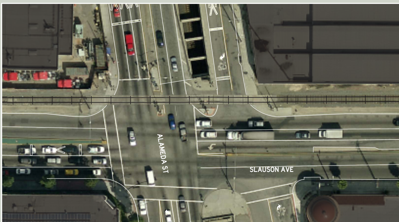
Figure 6 - Roadway Width: Signalized 60'-110' Crossing
