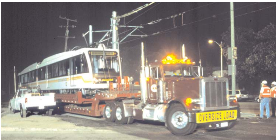
The first of six Metro Gold Line test cars is delivered alongside tracks in South Pasadena on a big-rig truck with an oversized trailer. Each car weighs 49 tons and is 89 feet long.
