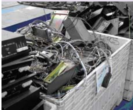
Incompatible PA systems and wiring were removed from all 69 Blue Line trains.
