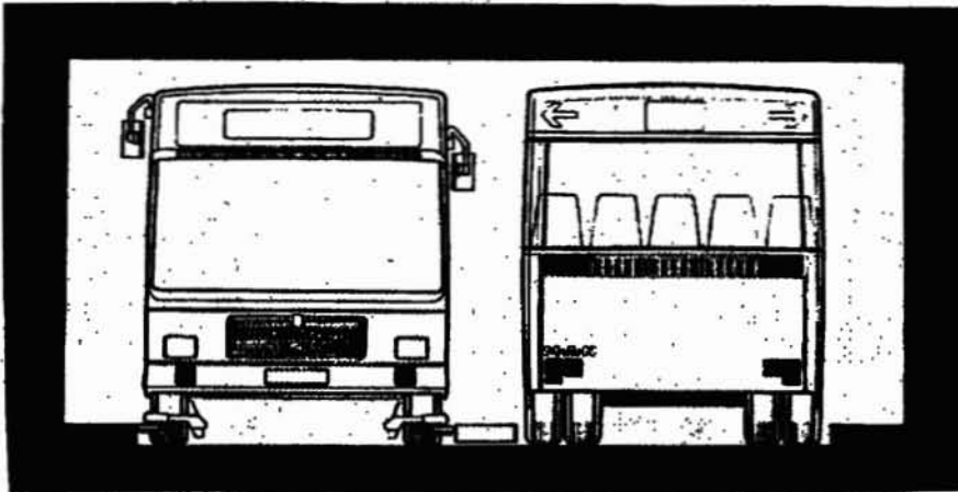
Left: The Spurbus and O-Bahn guideway bus systems rely upon rollers bearing upon lateral guide-rails for self-steering.
