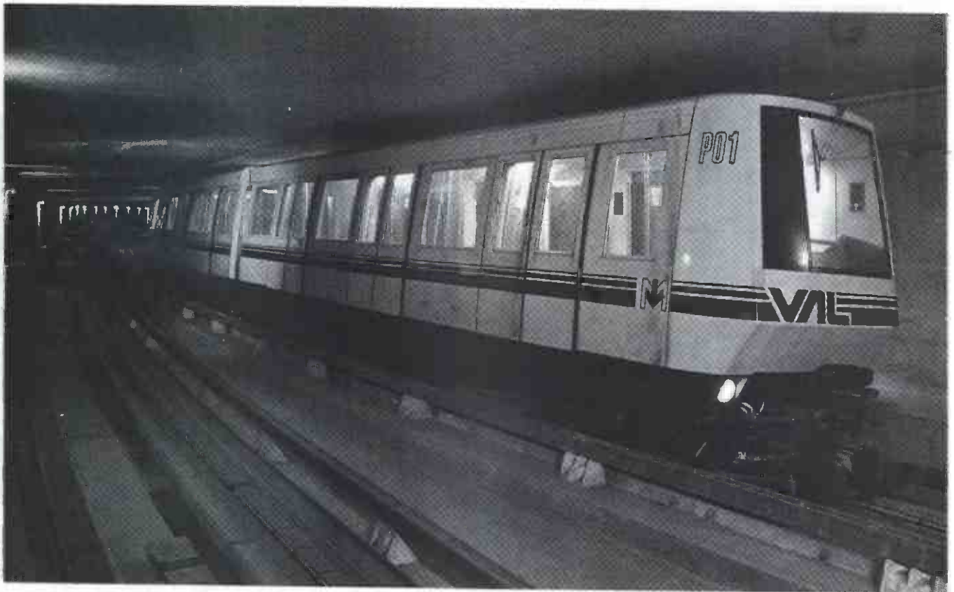
Lille is the site of the new VAL metro system, a fully automated operation.
