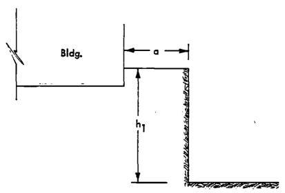
NOTE: Resultant of lateral pressure equals net building pressure  $x F x h_1^2$ . See text for explanation
