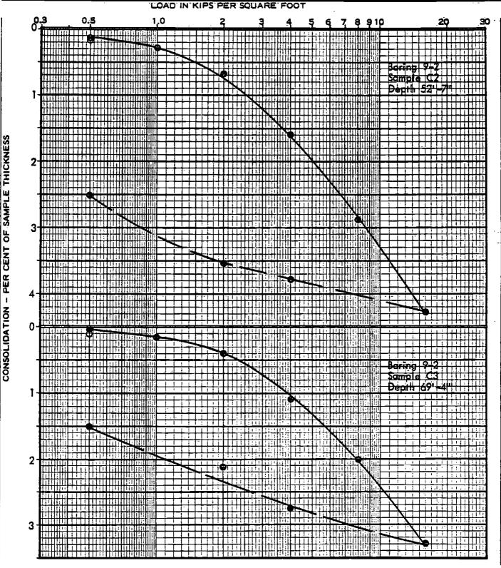
. READINGS AFTER SATURATION WITH WATER
