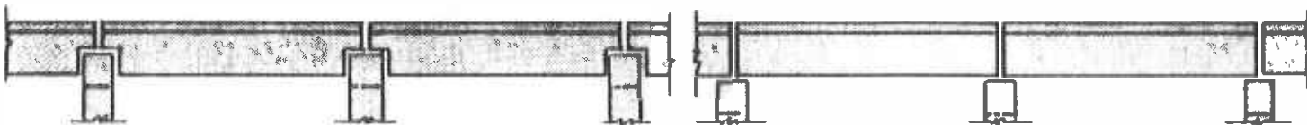
B. Simple Spans, Dapped Ends
