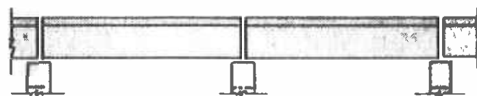
C. Simple Spans, Full-Depth Ends
