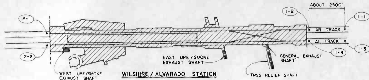
PROBE POINTS IN TUNNELS
