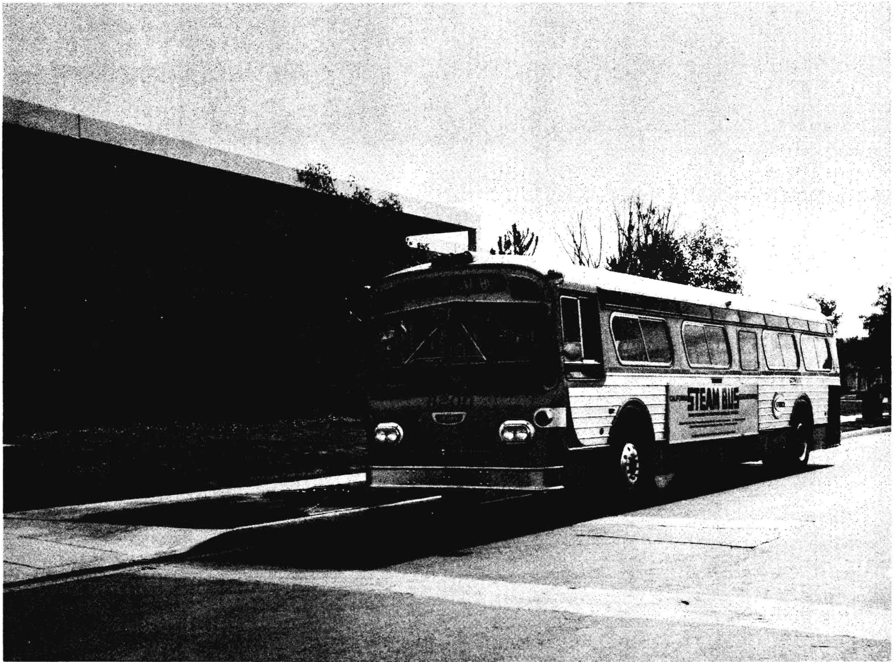
Fig. 1 - A forty foot urban coach converted to steam power. (Southern California Rapid Transit District, Power Plant by Steam Power Systems, Inc.)
