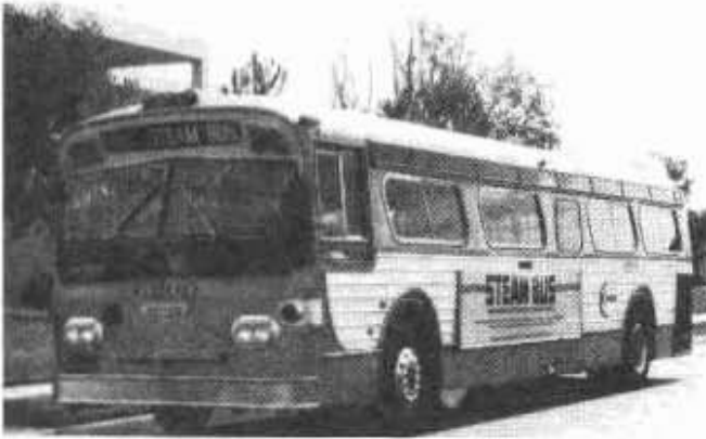
Fig. 1 - A 40 ft urban coach converted to steam power. (Southern California Rapid Transit District, with powerplant by Steam Power Systems, Inc. Illustration courtesy SPS, Inc.)
