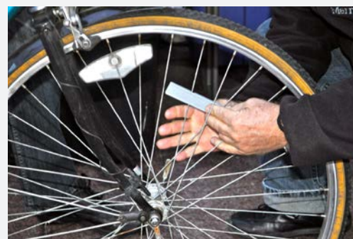
Installing the RFID tag in the bike wheel, for tracking and counting purposes; Zap Minneapolis and St. Paul.
