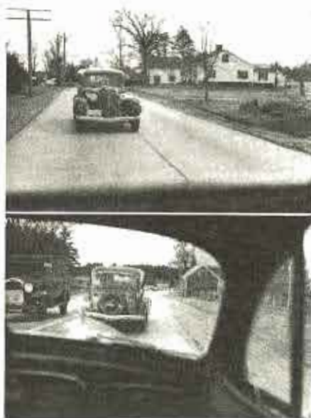
Figure 2. Flying Pass with Forced Return. Top—Start of Pass, View to Rear from Observation Vehicle. Bottom—Completion of Pass, View to Front Showing Forced Return Due to Counter Traffic.
