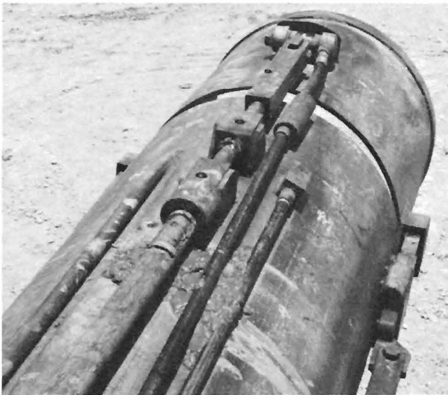
FIGURE 15 Finished LAG steering system for auger boring method.
