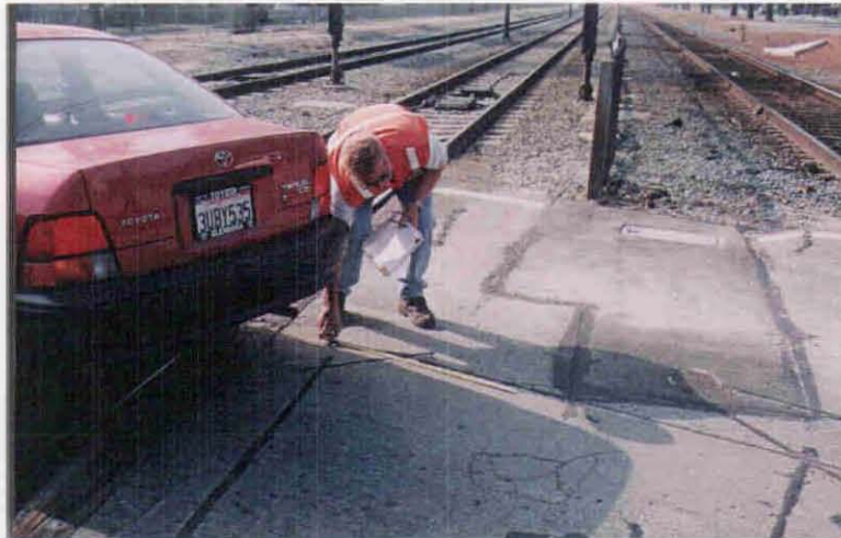
Figure 4-3 VERIFYING TRACK AREA VEHICLE DETECTION LOOP COVERAGE
