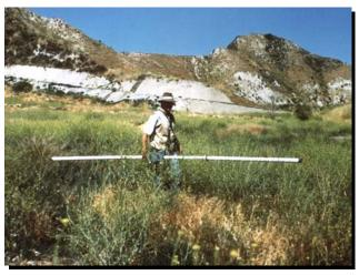
Geonics EM-31 Terrain Conductivity Meter
