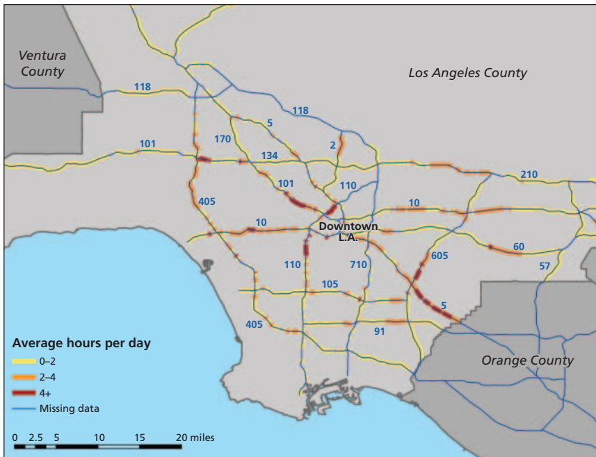
Figure S.3 Hours per Day During Which Freeway Speeds Average Less Than 35 mph in General-Purpose Lanes, 2006 Weekdays
