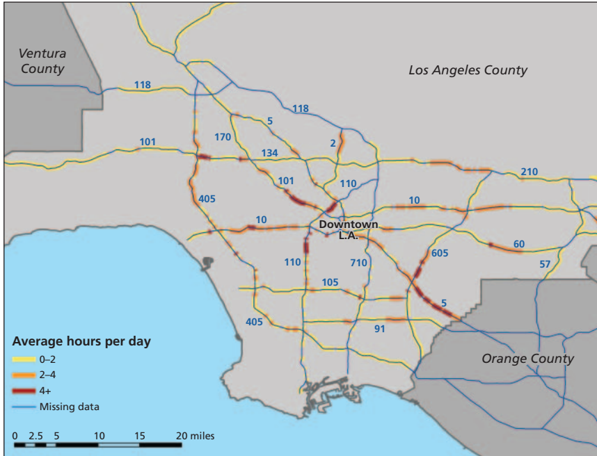
Figure 3.5 Average Hours per Day During Which Speed Averaged Less Than 35 mph in General-Purpose Lanes, 2006 Weekdays
