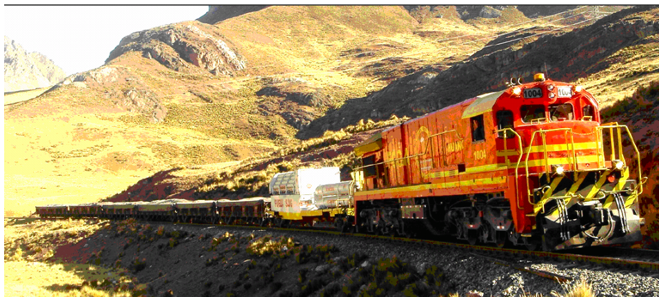
Figure 2: GE Natural Gas Locomotive
