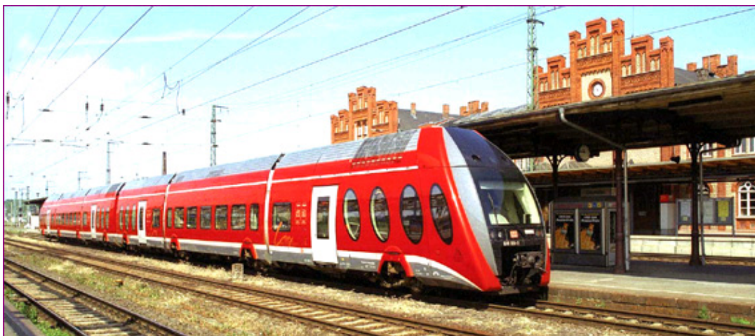
Figure 3: Alstom LIREX Experimental DEMU with Flywheel Storage
