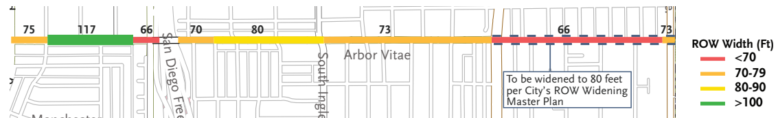
Source: AECOM Figure 2.1-10 Arbor Vitae ROW Widths
