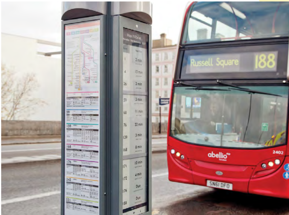
Kiosks in London equipped with reader-friendly e-ink display technology show bus arrival times. Photo courtesy of Technoframe.
