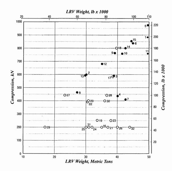
FIGURE 1 Compression versus LRV weight.
