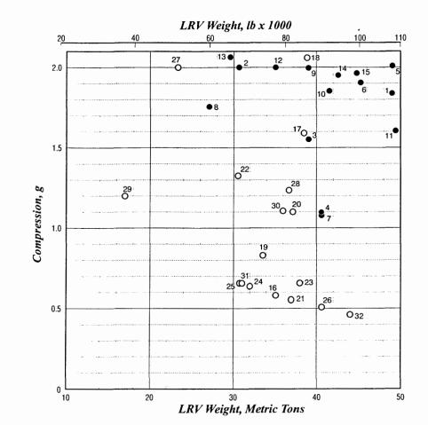
FIGURE 2 Compression in g's versus LRV weight.
