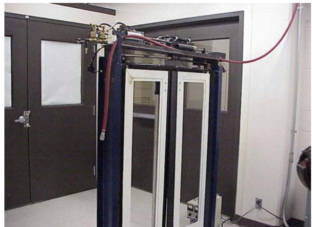
FIGURE 7 Door module allows training and diagnostic functions to be conducted in a classroom setting (source: DART).
