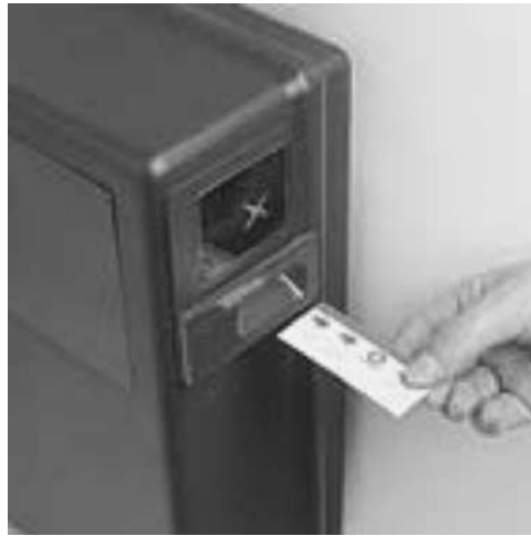
Figure 5-7: Adelaide Ticket Validator / Dispenser
