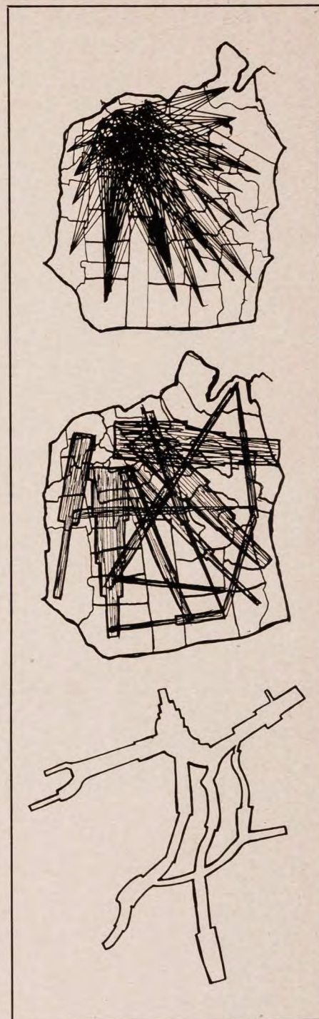
Graphic presentation of O & D results. Sequence: desire lines, major desire lines, and optimum location lines
