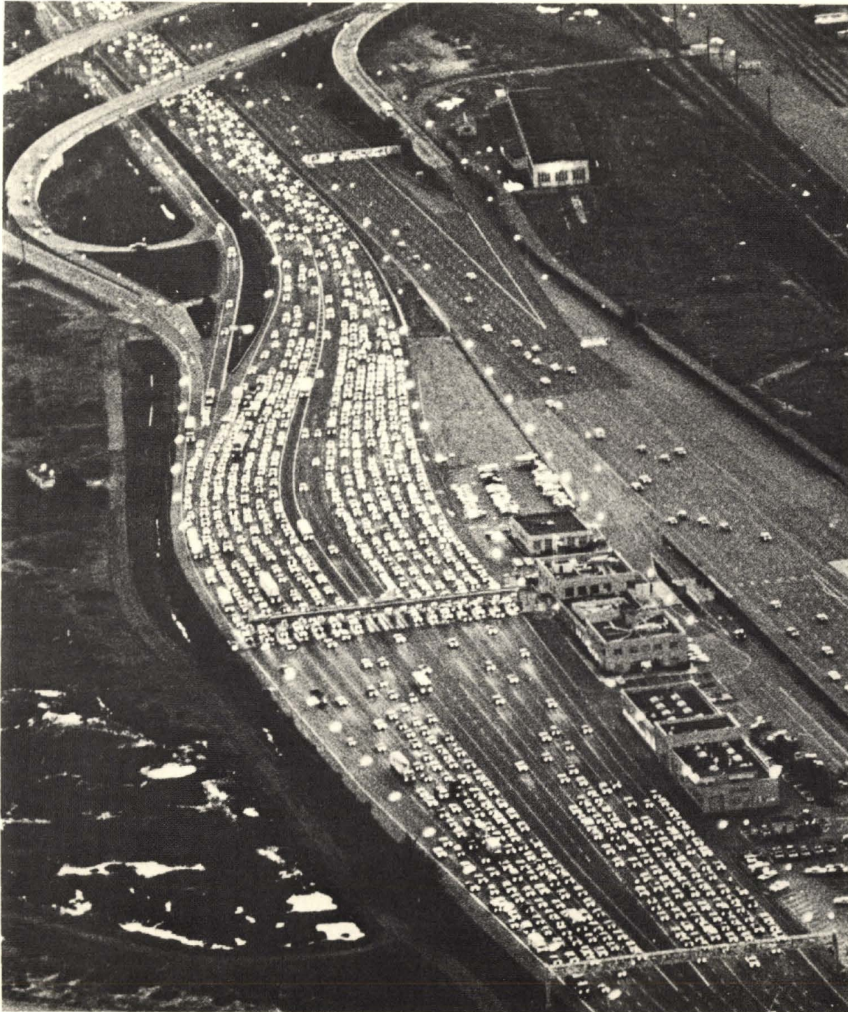
◀ San Francisco Bay Bridge toll plaza and metering signals, with HOV bypass lanes. (San Francisco Examiner.)
