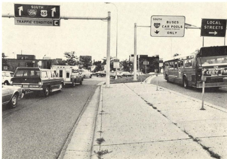
▲ Priority lanes provide preferential access to buses, carpools, and other priority vehicles. (Minnesota Department of Transportation.)
