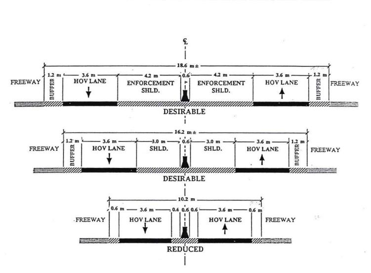
Recommended Two-Way Buffer-Separated Concurrent HOV Facility Cross Sections
