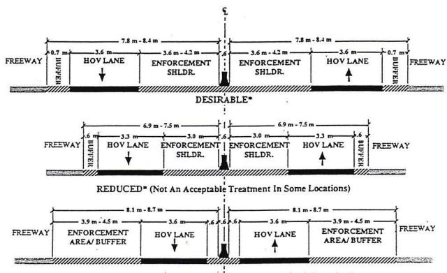
High-Speed Enforcement Areas along Two-Way Buffer-Separated HOV Facilities
