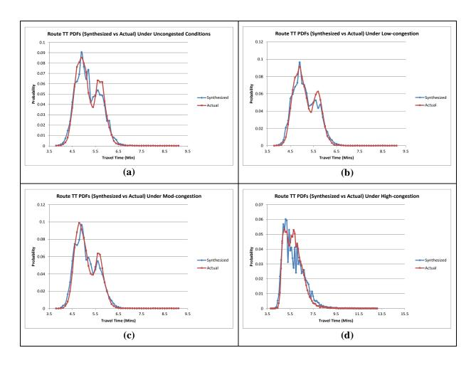
**Figure 6-12:** Comparisons between the travel time density functions synthesized from individual segment percentiles (squares) and the observed values (dots).
