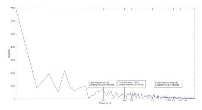
Figure 5-13: Frequency distribution for end-to-end travel time data along a freeway segment, based on the NGSIM data set
