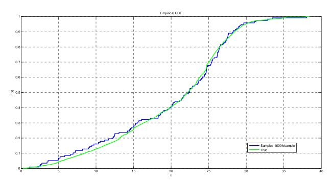
Figure 5-12: Reconstructed and ground truth traffic speed CDFs under sampling spacing of 2,000 ft/sample
