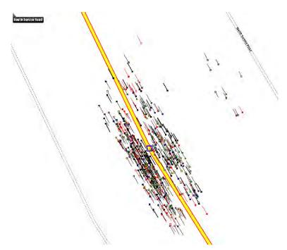
Figure 4-3: Locations and Headings Reported by AVL-Equipped Vehicles Trips Source: ALK Technologies
