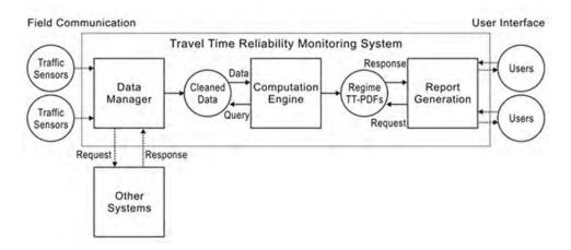
Figure 8-2: Block Diagram for a Travel Time Reliability Monitoring System (TTRMS)
