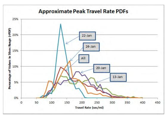
Figure 6-5: Peak Condition Travel Rates measured by Bluetooth Sensors for the Berkeley Highway Lab (segment length of about 4500 feet)
