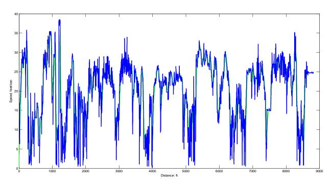
Figure 5-9a: Reconstructed speed time series for GPS traces under cutoff frequency of 1,000 ft/sample
