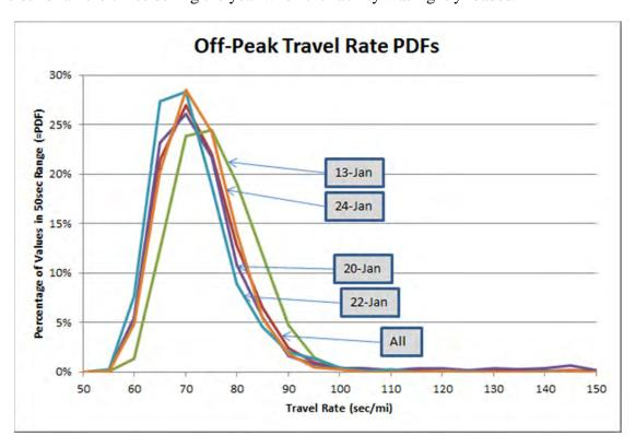
Figure 6-4: Off Peak Travel Rates measured by Bluetooth Sensors for the Berkeley Highway Lab (segment length of about 4500 feet)
