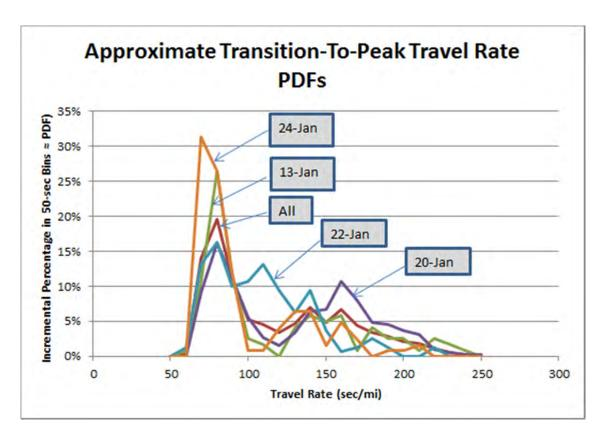
Figure 6-6: Transition to Peak Condition Travel Rates measured by Bluetooth Sensors for the Berkeley Highway Lab (segment length of about 4500 feet)
