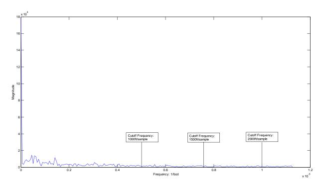
Figure 5-8: Frequency domain representation for GPS location-based speed data along space dimension
