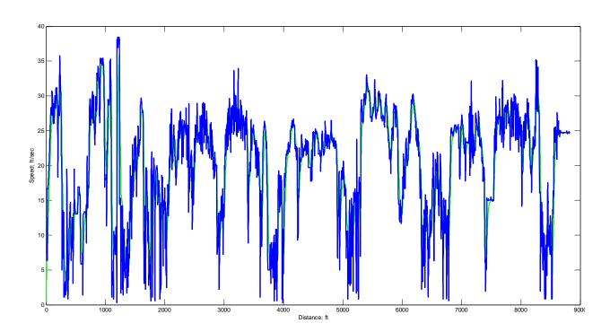
Figure 5-9c: Reconstructed speed time series for GPS traces under cutoff frequency of 2,000 ft/sample
