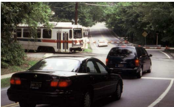
A crossing controlled by automatic gates on Philadelphia's LRT system.
