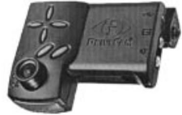
DriveCam—a palm-sized video data recorder that mounts behind a vehicle's rearview mirror and continuously monitors driving activity—is an example of the innovative research projects supported by Division E.
