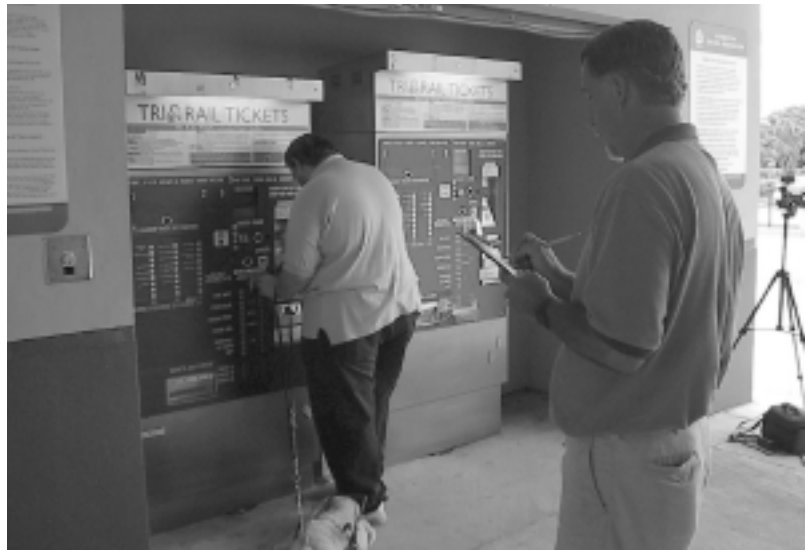
Transit IDEA program supervised the testing of an audio-enhanced ticket machine for transit riders with impaired vision.
