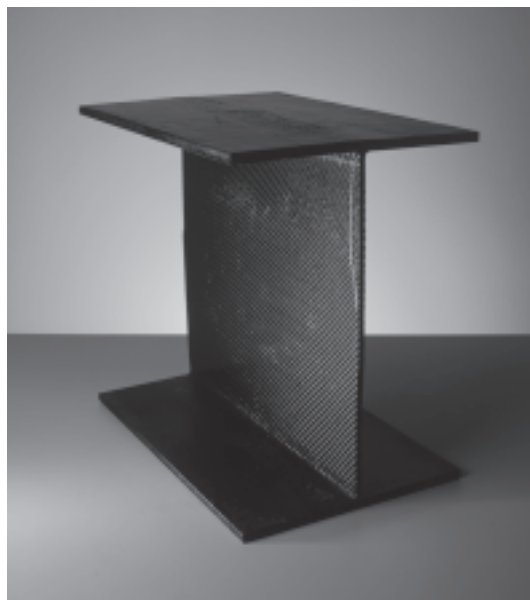
Carbon fiber I-beam, developed through NCHRP-IDEA Project 67 for lightweight sidewalks on roadway bridges, was displayed as an example of inventive engineered fabrics at the Cooper-Hewitt National Design Museum in New York.
