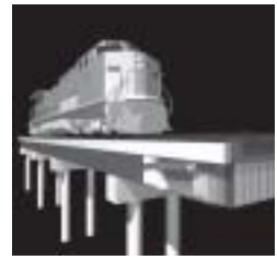
Three-dimensional representation of the hybrid-composite bridge beam, developed by John Hillman of Teng and Associates with support from the TRB IDEA Program. Now patented, the beam is a revolutionary new type of structural member for bridges, offering improved corrosion resistance and service life.
