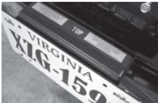
Instrumentation for the SHRP 2 naturalistic driving study will include radar sensors mounted behind the license plate. (Photo courtesy of Virginia Tech Transportation Institute.)
