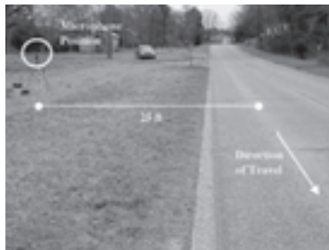
Pass-by noise measurement setup for a portland cement concrete test site in Waverly, Alabama, from NCHRP Report 630, Measuring Tire-Pavement Noise at the Source .
