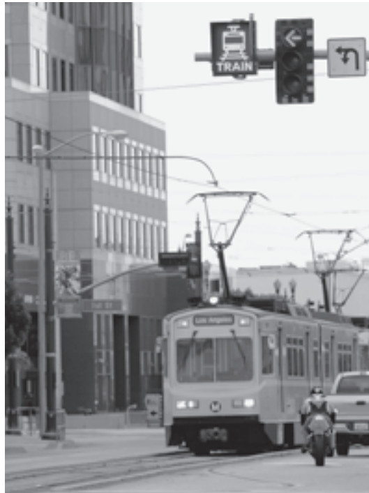
A train-activated warning sign in Los Angeles, from TCRP Synthesis 79, Light Rail Vehicle Collisions with Vehicles at Signalized Intersections .
