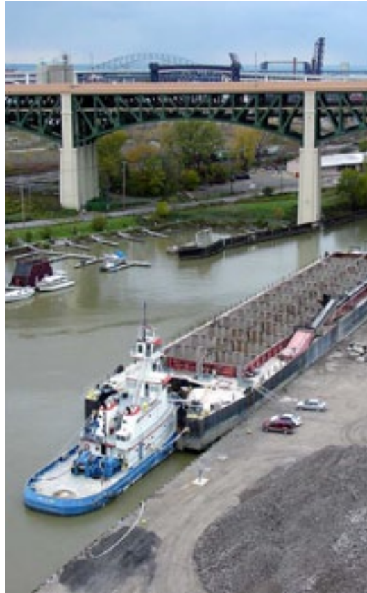
Integrated tug-barge units, widely used in Gulf of Mexico and East Coast offshore trade, are examined in National Cooperative Freight Research Program Report 5, North American Marine Highways .
