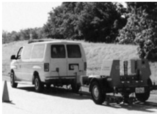
A trailer-mounted falling weight deflectometer was one of the nondestructive testing (NDT) devices assessed in NCHRP Report 626, NDT Technology for Quality Assurance of Hot-Mix Asphalt Pavement Construction .
