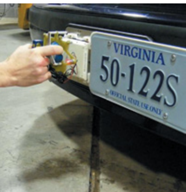
Installation of a prototype of the forward radar assembly, which gathers data from the vehicles of the participants in the Naturalistic Driving Study (NDS). (Photo: SHRP 2)
