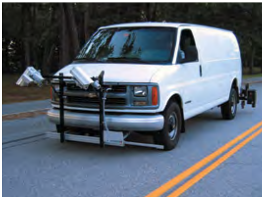
A vehicle-mounted unit for measuring the reflectivity of pavement markings was developed by Terry Lee with support from NCHRP IDEA. (Photo: Terry Lee)
