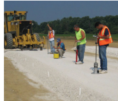
NCHRP Synthesis 456 examines national and international experience with nonnuclear devices and methods for measuring compaction of unbound materials. (Photo: Iowa State University, 2008)
