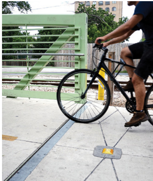
Inductance loops and infrared sensors on Lance Armstrong Bikeway in Austin, Texas, along with other traffic counting technologies, were presented in Transportation Research Circular E-C183, Monitoring Bicyclist and Pedestrian Travel and Behavior . (Photo: Jim Lyle, TTI)
