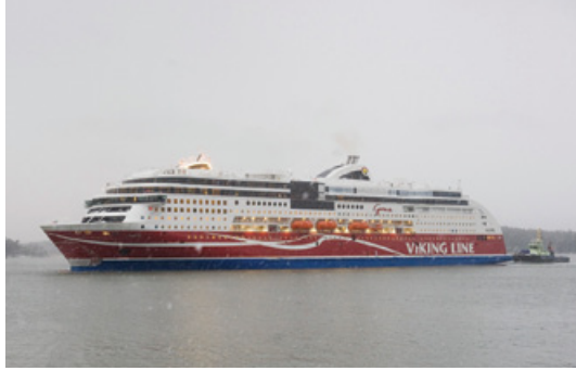
The MS Viking Grace is the first large-scale passenger ferry to be powered by liquefied natural gas (LNG). Issues related to vessels powered by LNG were on the agenda at the Marine Board's fall meeting. (Photo: Meyer Turku Oy)
