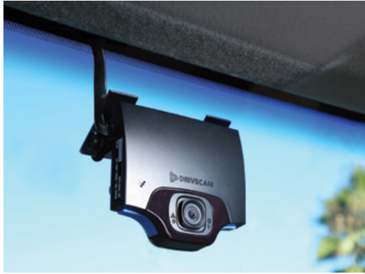
Lytix—formerly DriveCam—developed the widely used DC3P Video Event Recorder, which received seed funding and early testing through TRB’s Intelligent Transportation Systems IDEA program. (Photo: Lytx, Inc.)
