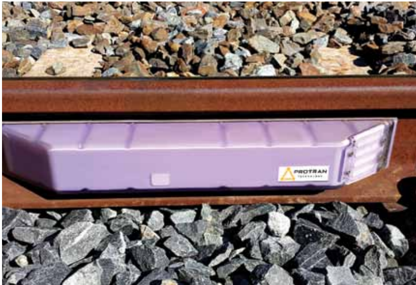
Protran's Rail Neutral Temperature Monitoring system, first developed with support of the Transit IDEA program, monitors the health of continuous rails. (Photo: Protran)
