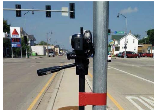
An NCHRP IDEA project examined the use of available vehicle detection devices for automated counts of turning movements in shared lanes. (Photo: Kelvin R. Santiago)
