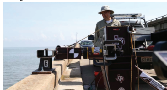
Research presented at the first International Roadside Safety Conference included full-scale testing of retrofit bridge rails for causeway bridges over Lake Pontchartrain in Louisiana. (Photo: William F. Williams, Texas A&M Transportation Institute)
