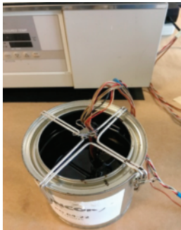
Duomorph asphalt rheology tester (top) and test setup (bottom). Developed under NCHRP IDEA Project 193, the low-cost, piezoelectric sensor-based portable testing system monitors the quality and specification compliance of asphalt binder samples at various points along its supply chain. (Photos: Cooperative Research Programs)
